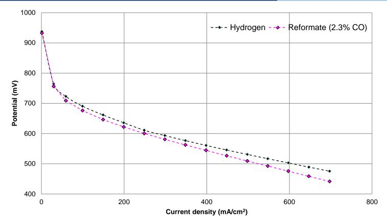
Polarization curve for MEAs tested with hydrogen and reformate at 160 °C ( $\lambda_{H2}$ =1.25,  $\lambda_{air}$ =2.5 and ambient pressure).
