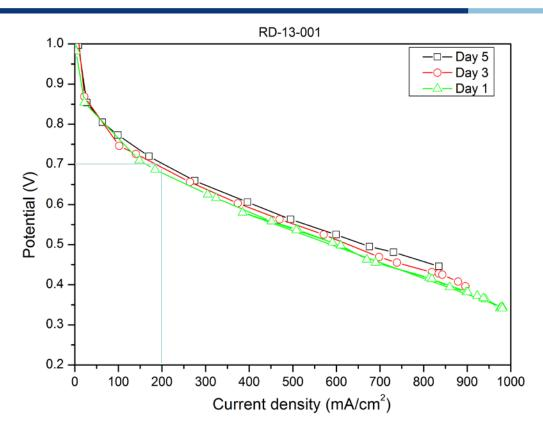
Polarization curves at 160 °C 49 cm<sup>2</sup> MEA. The Pt loading on the cathode 1.5 mg Pt/cm<sup>2</sup> (JM HiSpec9100) The MEA's was measured by AAU.
