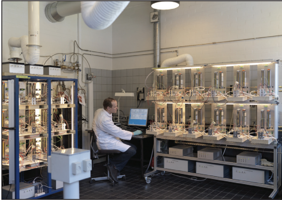
The 2x12 channel fuel cells durability rig
