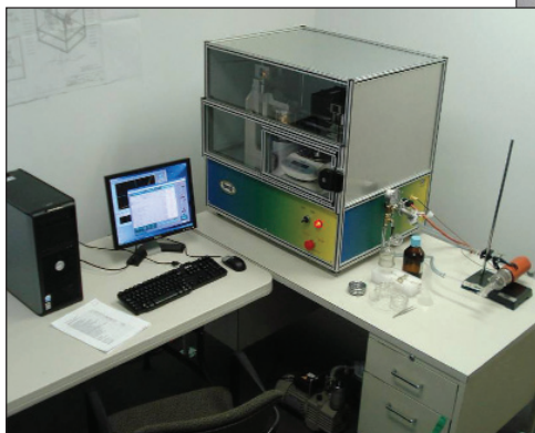
Porosimeter for detailed characterization of porous transport media
